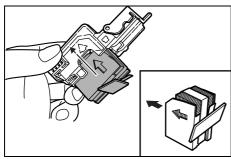
**4** Holding the staple holder in your left hand, insert a new staple case with your right hand in the direction of the arrow.
